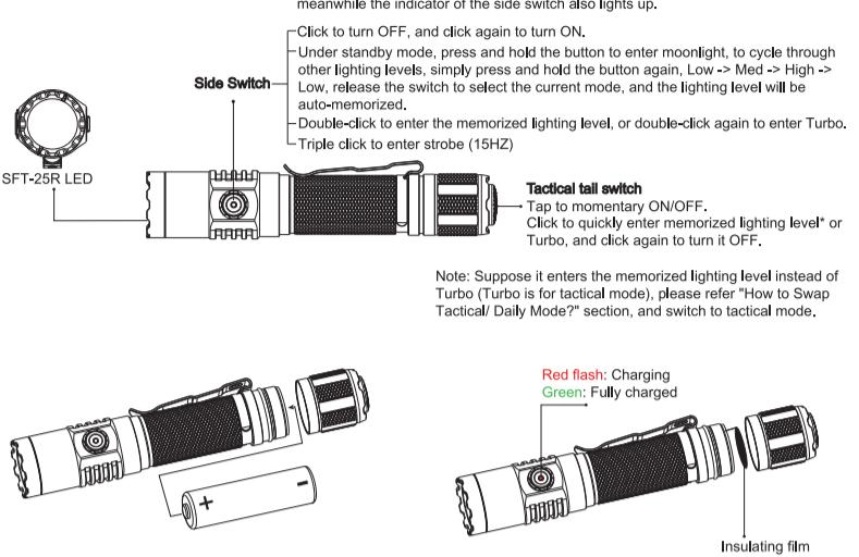
Note: Before pushing the side switch, be sure to press the tail switch first to turn it on, meanwhile the indicator of the side switch also lights up.
